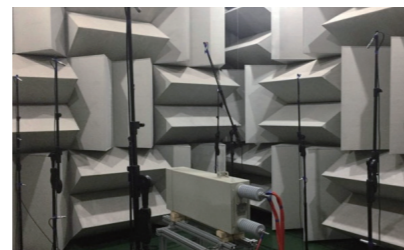
Capacitor noise test room
