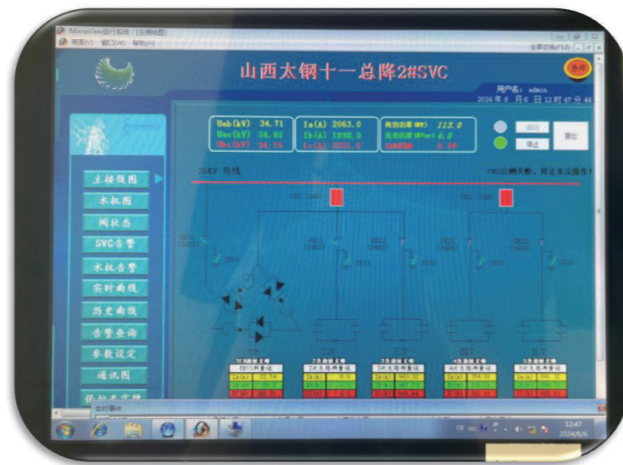
Diagram of the 200 MVar/35 kV SVC Unit of Taiyuan Iron & Steel (Group) Co., Ltd. in Shanxi
